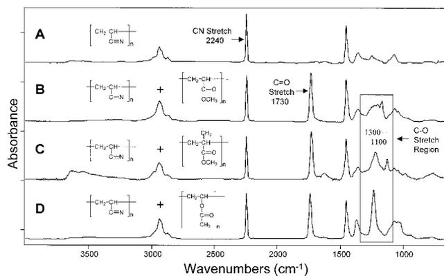
FIG. 5. Comparison of infrared spectra of four major acrylic sub-generic classes. (A) polyacrylonitrile homopolymer; (B) poly(acrylonitrile:methyl acrylate); (C) poly(acrylonitrile:methyl methacrylate); (D) poly(acrylonitrile:vinyl acetate).
