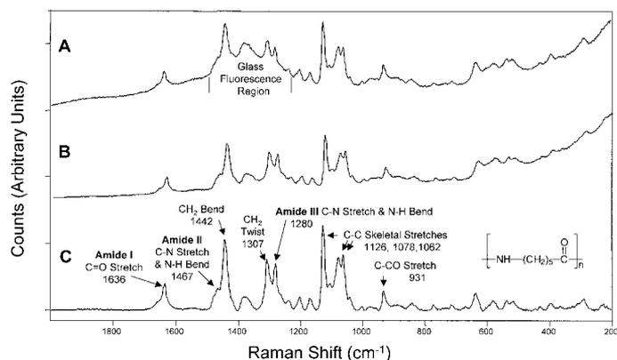
FIG. 1. Raman spectra of a nylon 6 fiber on different mounts. (A) nylon 6 taped on a glass slide; (B) nylon 6 taped on an aluminum foil slide; (C) nylon 6 on an aluminum foil slide after baseline flattening.
