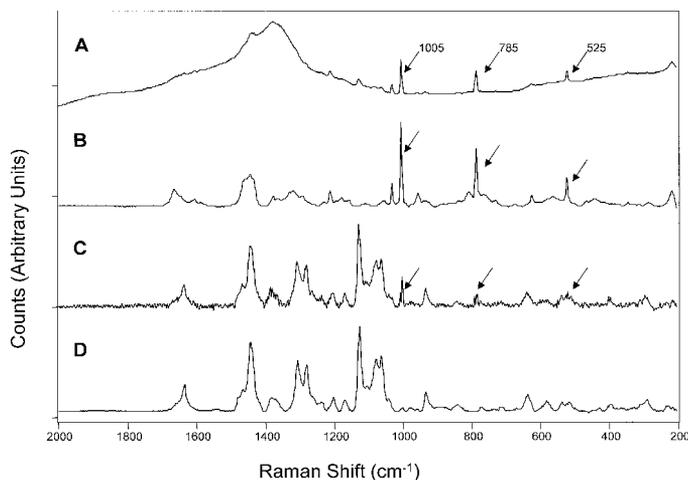
FIG. 2. Raman spectra of a nylon 6 fiber mounted on a glass slide in Permout with a coverslip. (A) nylon 6 mounted in Permout (arrows show major Permout peaks); (B) Permout on aluminum foil; (C) nylon 6 mounted in Permout after subtraction of Permout and glass slide and baseline flattening plotted full scale (arrows show subtraction artifacts); (D) nylon 6 spectrum obtained on aluminum foil-covered slide.
