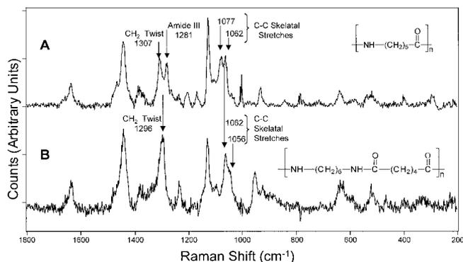
FIG. 3. Comparison of Raman spectra of two nylon fibers mounted in Permount with the distinguishing peaks labeled. (A) nylon 6; (B) nylon 6,6.
