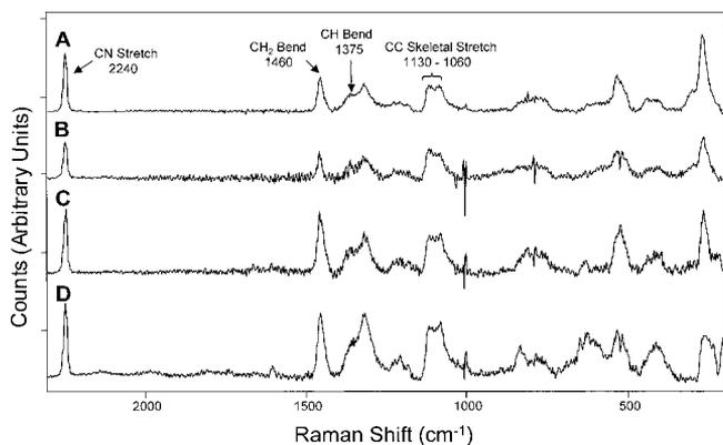
Fig. 6. Comparison of Raman spectra of four major acrylic subgeneric classes. (A) polyacrylonitrile homopolymer; (B) poly(acrylonitrile:methyl acrylate); (C) poly(acrylonitrile:methyl methacrylate); (D) poly(acrylonitrile:vinyl acetate).
