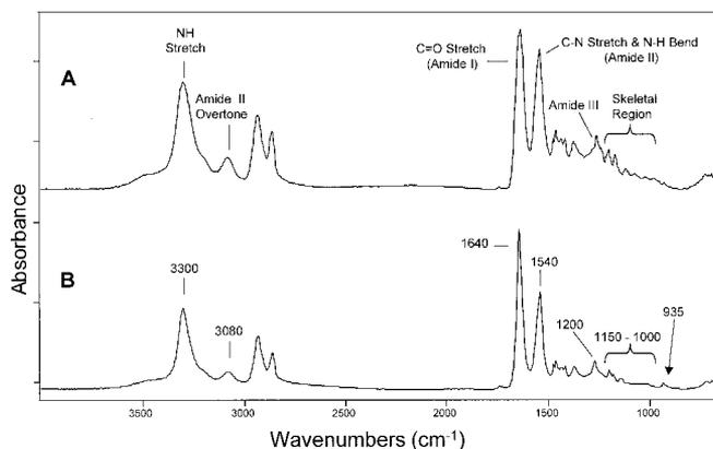
FIG. 4. Infrared spectra of two nylon fibers with the distinguishing peaks labeled. (A) nylon 6; (B) nylon 6,6.
